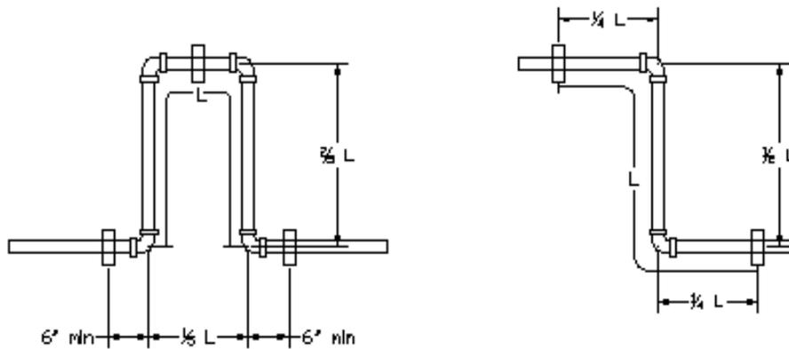
The minimum calculated length of offset may be distributed as segments of a loop or other means for imparting flexibility. Recommended minimum lengths for each segment are illustrated above.  $L$  is the total offset length as determined by means of Equation 5.
