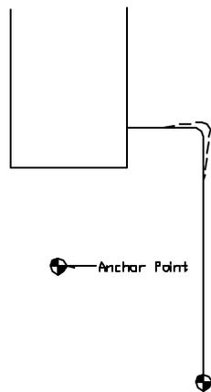
In this layout, thermal expansion of the longer vertical run results in the development of high bending stresses in the shorter horizontal run.
