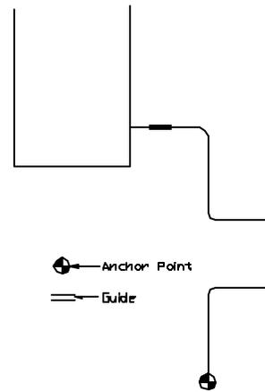
Two techniques for isolating a short branch from excessive bending are shown by the use of a loop, which safely absorbs the vertical expansion, and by the placement of a guide, or support, in the short horizontal run to protect it against bending.
