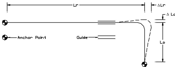
A pipe offset relieves an axial thrust by transforming it into a moderate bending stress.
