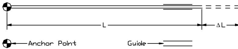
A pipe anchored at one end will expand in length when subjected to a higher temperature.
