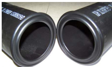
Figure 2 - Unacceptable Concave Melt Appearance
