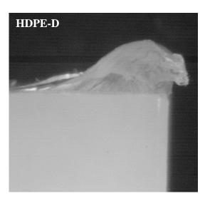
In Figure 5, the stretched portion of the PENT specimen is shown; this picture was taken on a specimen after the test was stopped prior to ultimate failure. This is another clear indication that post-yield tensile stretching (ductile fracture) exerts a considerable influence on the PENT failure time.
