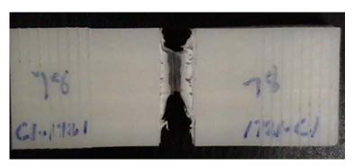
The PENT failure times encompass the time-scale for fracture initiation, crack propagation and post-yield tensile stretching. The brittle fracture of pressurized polyethylene pipes does not include a macroscopic ductile component. Therefore, it is perhaps not surprising that there is no correlation between PENT and brittle fracture of pressurized polyethylene pipes.
