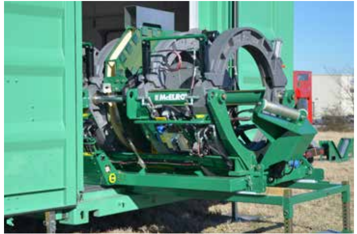
Fusion carriage can be removed for in-ditch use or fusing of stub ends and fittings.
